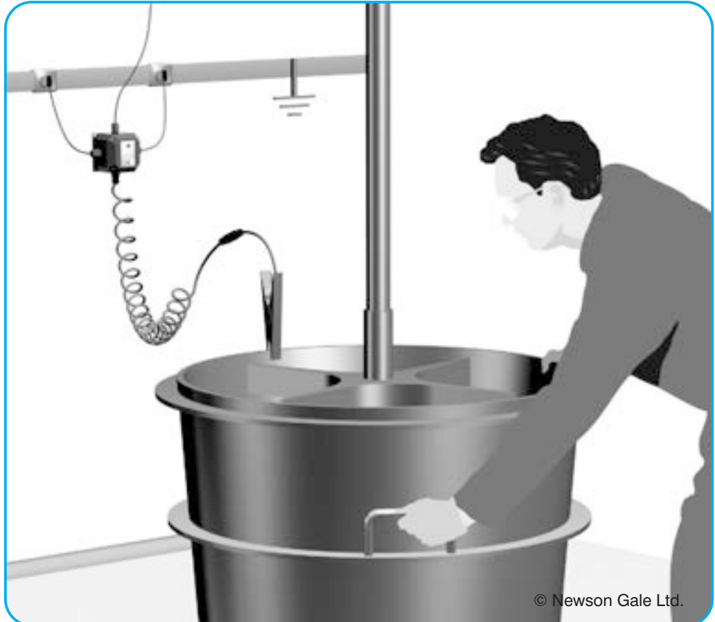
Close up of Earth-Rite TELLUS II Intrinsically Safe Indicator Station.
